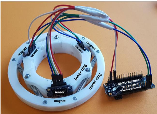
Fig. 1: Prototype of KRIS (Kinesthetic Robotic Interaction System).
