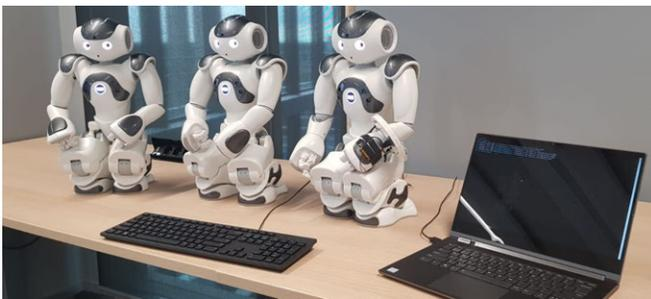
Fig. 5: User study setup. The left NAO is used to indicate the target pose in the Pose Mimic experiment, the middle NAO is used as baseline with the keyboard and the right NAO is mounted with KRIS.
